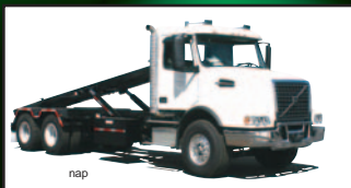
2003 VOLVO ROLL-OFF 365 H.P. VE-D12 ENGINE, 8 SPD TRANSMISSION, 44,000 LB. REARS, 60,000 LB. GALBREATH ROLL-OFF HOIST. (F393) ..... $95,900
