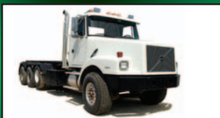
1997 VOLVO ROLL-OFF 330 H.P. M-11 ENGINE, 8SPD TRANSMISSION, 56,000 LB. REARS, 60,000 LB. GAL-FAB ROLL-OFF HOIST. (G089) ..... $64,900
