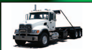
2006 MACK GRANITE ROLL-OFFS 405 H.P. MACK ENGINE, 8 SPD TRANSMISSION, 44,000 LB. REARS, 60,000 OR 75,000 LB. GALBREATH ROLL-OFF HOIST, LOADED WITH EXTRA FEATURES. STARTING AT $114,900
